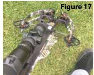
5. To release any tension in the cocking system, rotate the draw handle slightly forward toward the top of your Ravin Crossbow. Press the spool thumb release (Figure 18) then rotate the draw handle backward to release the tension.
