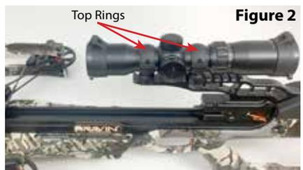
2. Lay the scope into the bottom rings. Place the top rings on the bottom rings so the scope is surrounded (Figure 2). Lightly snug up the screws on the top rings so you can still freely move the scope in the rings.
