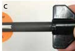
d. Place the Nock Installation Tool on a table top, and with two hands grasp the arrow shaft, near the fletching, and push downward until the nock is flush with the nock bushing. After you have fully installed new nock, make sure the pointer on the Nock Installation Tool is still aligned with the white cock vane.
