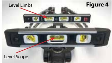
5. Remove the elevation turret cap and place a level on the elevation turret. Rotate the scope in the rings until it is level with your Ravin Crossbow limbs (Figure 4). The horizontal reticle markings should be parallel with your Ravin Crossbow limbs.
