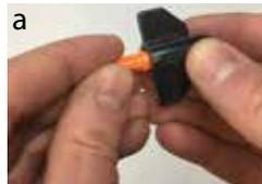
b. Locate the aluminum nock bushing at the rear of the arrow. Press the new nock into the nock bushing until the nock is tight and can't go any further. Do not use pliers to insert the new nock or you may damage the nock. Do NOT glue the nock into the bushing.
