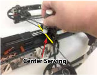
**5. Cold Weather Operation:** Apply a Ravin-approved **non-wax** lubricant to the center serving of the bowstring before operating your Ravin Crossbow. A suitable **non-wax** lubricant is Ravin Serving Fluid or Scorpion Venom™ Polymeric Bowstring Fluid.
