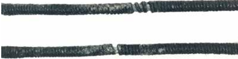
Examples of worn, damaged or separated center serving strings
